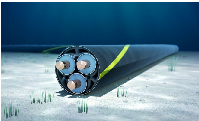
Underwater power cable (schematic illustration).
